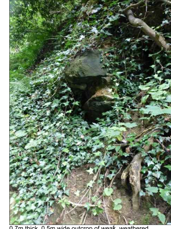
0.7m thick, 0.5m wide outcrop of weak, weathered sandstone 1.6m above the carriageway
